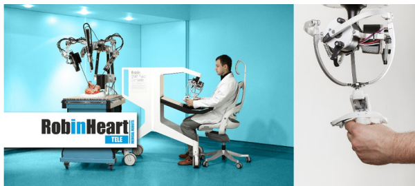
A. Robin Heart Tele and original, patented robot motion controller with force feedback
