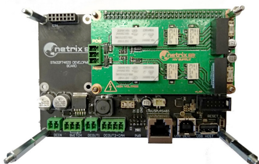
Figure 5. Assembled high-voltage inverter on the control module board
