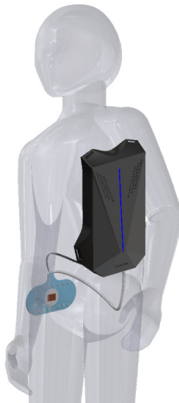
Figure 2. Visualization of a portable ultrasound-impedance tomograph with a sensor on the body
