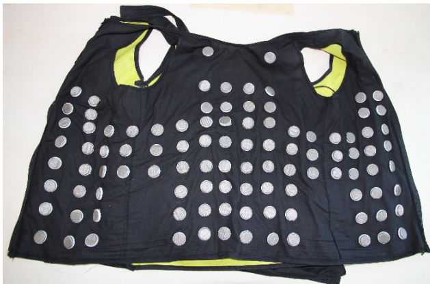
Figure 1. Developed vest with 102 textile electrodes
