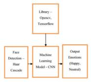
The dataset is used to train a neural network model. The pre-processing stage includes image visualization. The Panda's Python library is used for data analysis.
