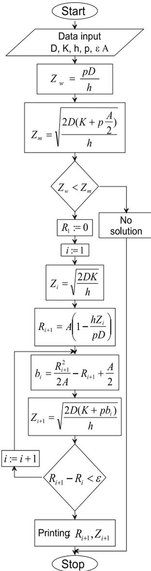
Figure 4.  $R_0$  and  $Z_0$  optimal values searching block diagram with uniform distribution
