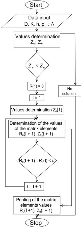
Figure 3.  $R_0$  and  $Z_0$  optimal values searching block diagram
